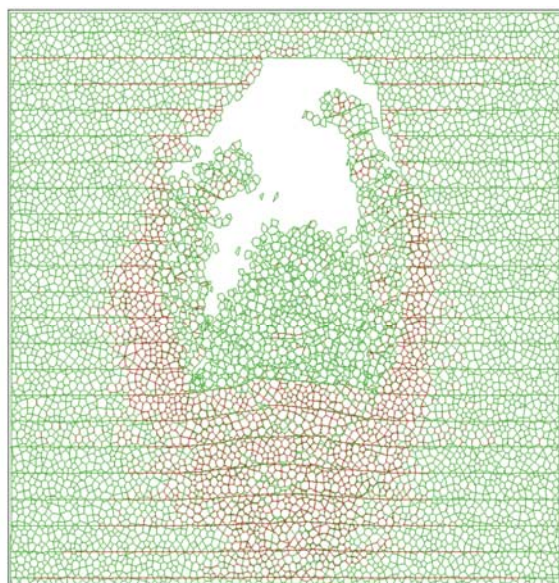
b) ground motion M5.5 at 15 km
